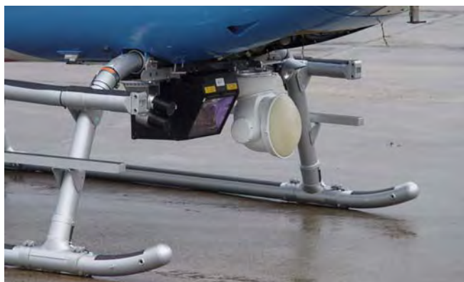
Figure 3: Sensor mounting between the landing skid.
