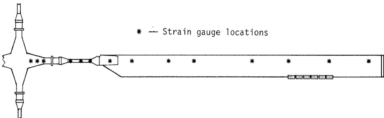
Fig 8 Strain gauge blade planform
