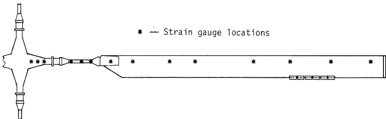
Fig 8 Strain gauge blade planform
