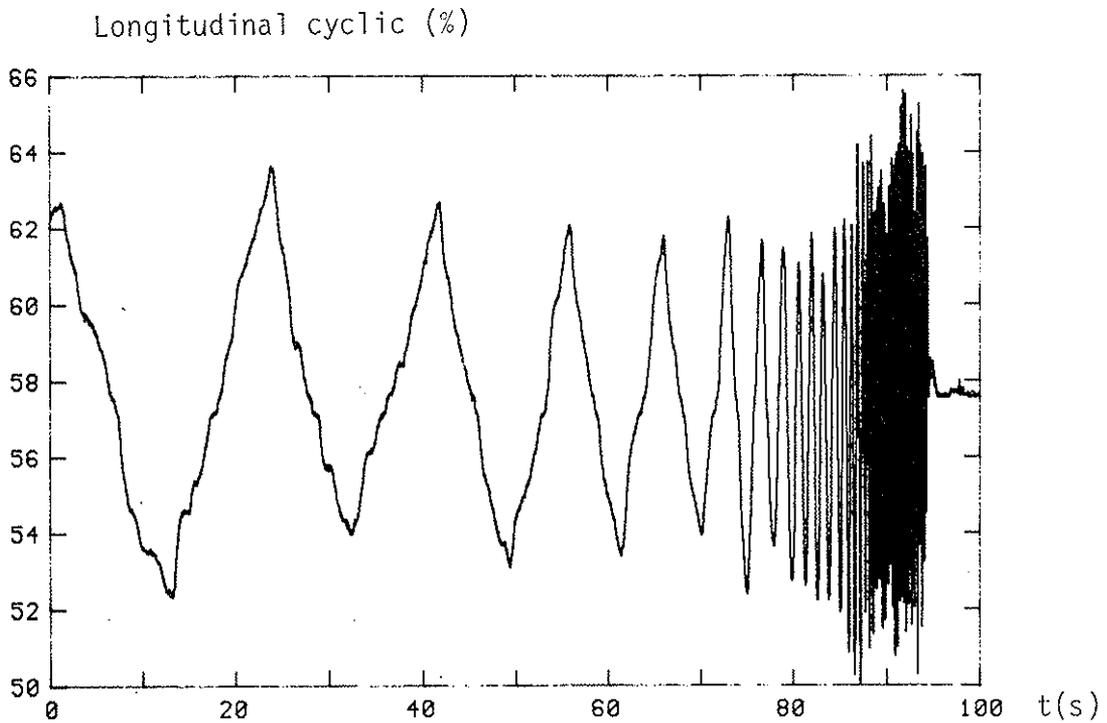
Fig 10 Lynx ZD559 - longitudinal cyclic frequency sweep
