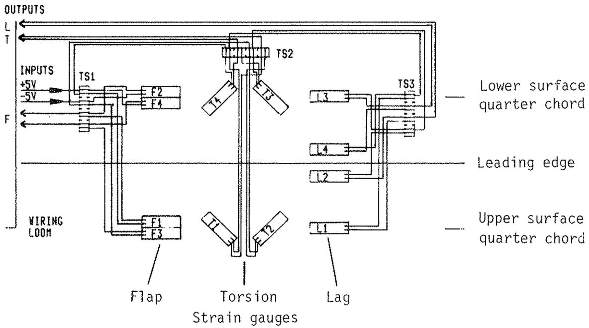
Fig 9 Strain gauge layout for each radial station
