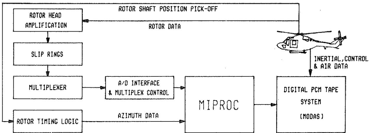
Fig 3 Schematic of data acquisition on research Lynx
