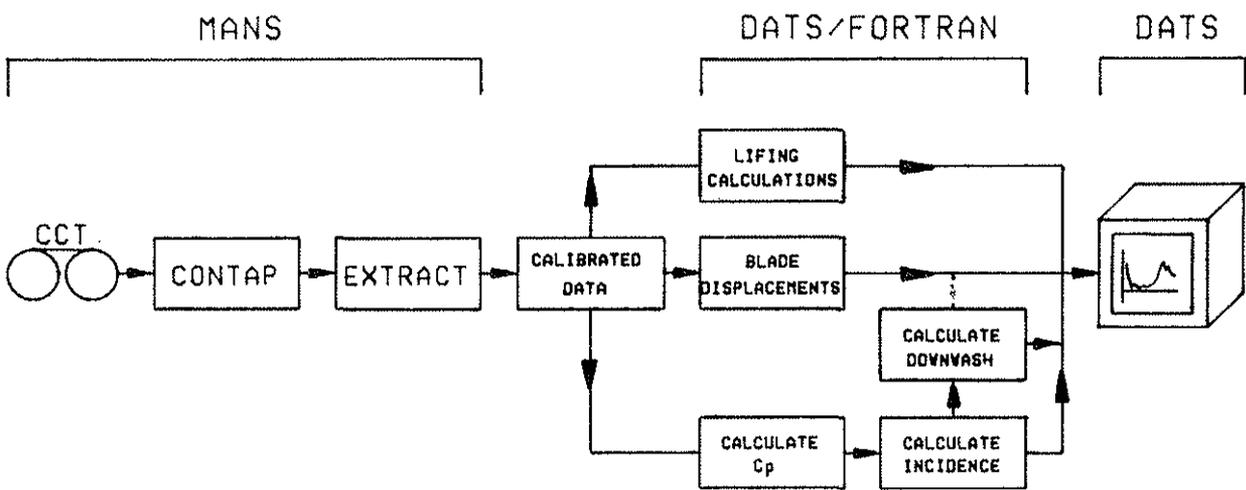
Fig 12 Elements of RIBAN package
