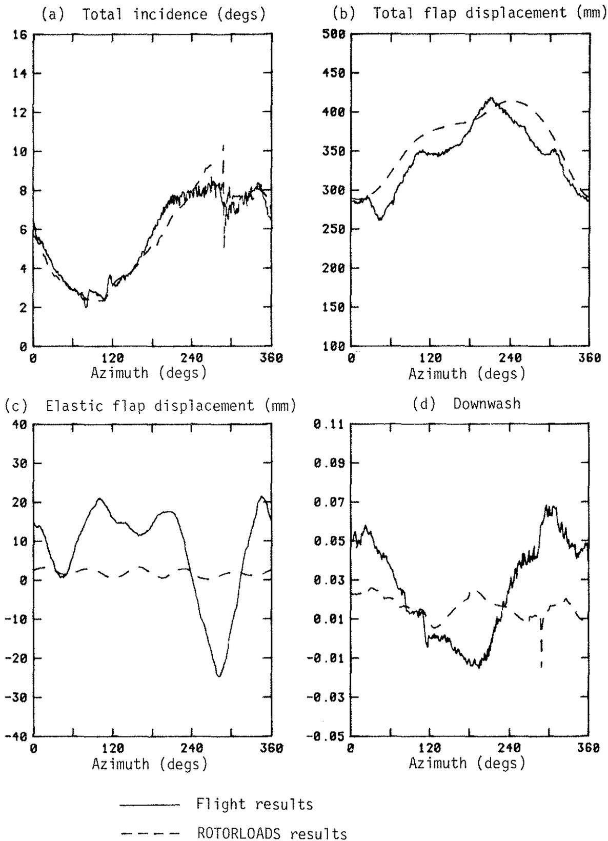
Fig 13 Puma XW241 - comparison between flight results and theory
