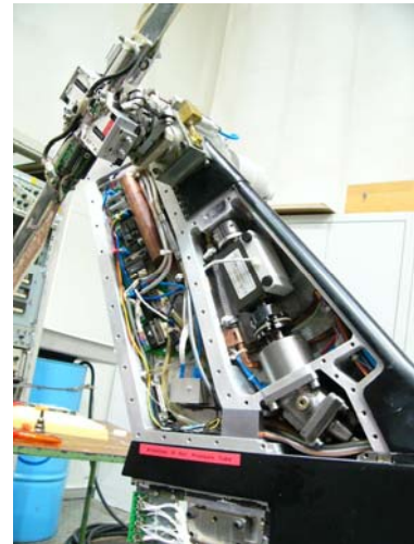
Figure 7 Tail fin with integrated tail rotor
