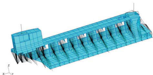
FIG. 3. Cut-away plot of the fuselage model exposing the RBE3 constructs (black spider webs) used for concentrated mass attachment to the frame/skin.
