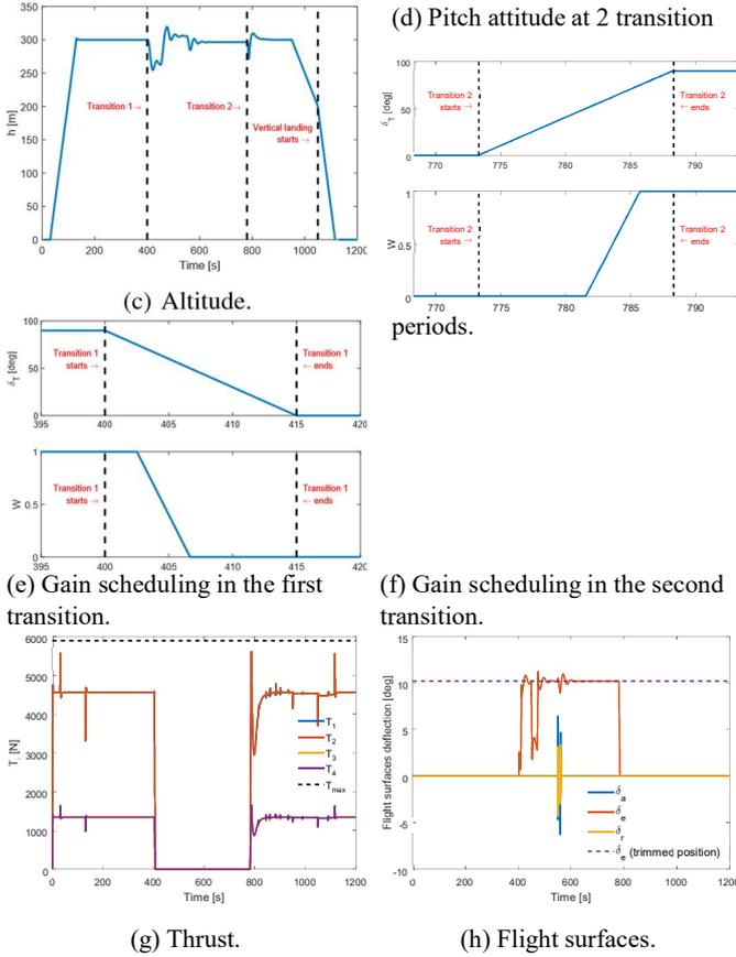
Fig. 18: Nonlinear simulation results for whole flight test.
