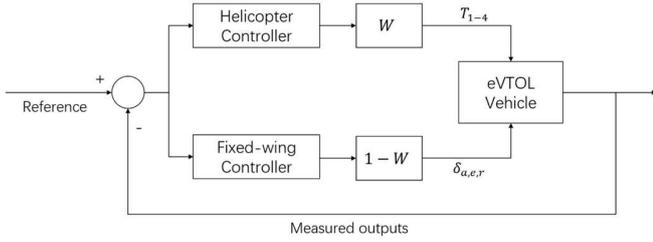
Fig. 11: DC gain scheduling structure for transition control.
