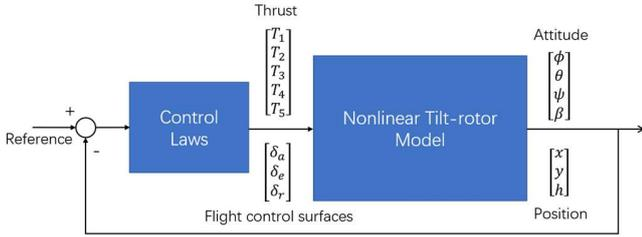
Fig. 4: Control diagram for the nonlinear tilt-rotor model.
