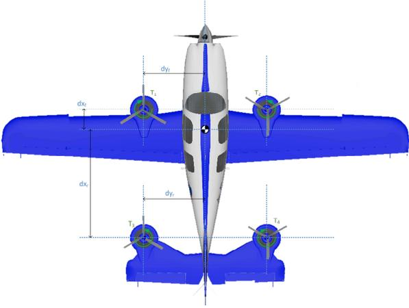
Fig. 3: Geometry information of the model [1].
