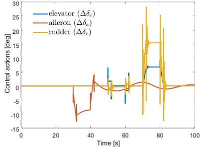
Fig. 16: Control actions (airplane mode). are
