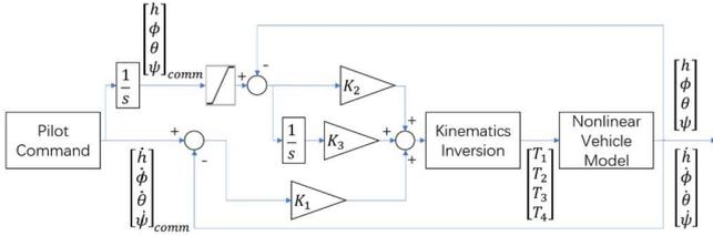
Fig. 5: Attitude and height control diagram in the helicopter mode.
