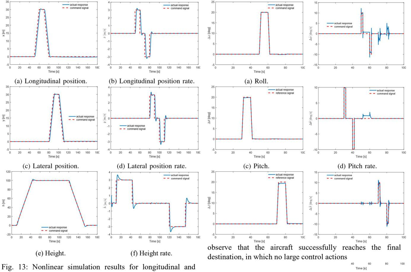
Fig. 13: Nonlinear simulation results for longitudinal and lateral position control (helicopter mode).
