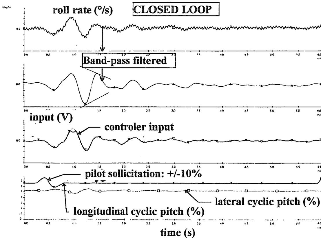
**Fig. 6: ACTIVE CONTROL FOR AIR RESONANCE - TIME DOMAIN**
