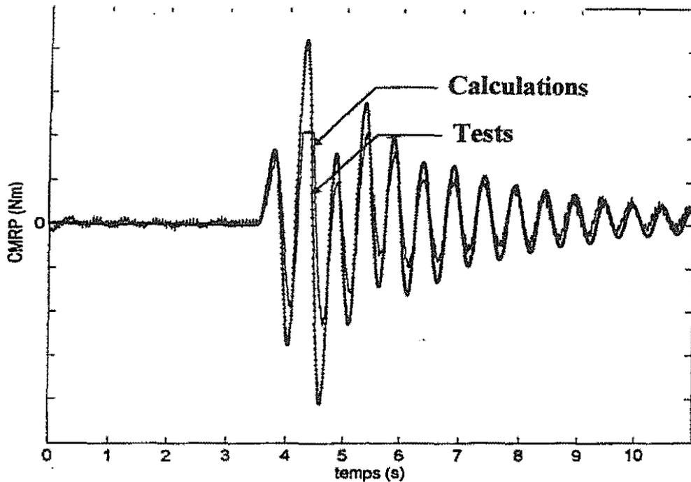
**Fig. 10: DRIVE TRAIN MODE IDENTIFICATION, CALCULATIONS/MEASUREMENTS COMPARISON**
