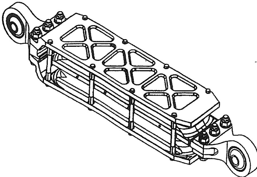
**Fig. 3: EXAMPLE OF VISCOELASTIC TECHNOLOGY DAMPER TO TESTING GROUND AND AIR RESONANCE ACTIVE CONTROL**
