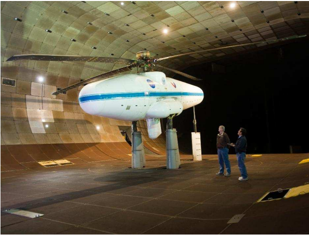
Fig. 1. Full-scale UH-60A rotor installed on the Large Rotor Test Apparatus in the NFAC 40- by 80- ft wind tunnel.
