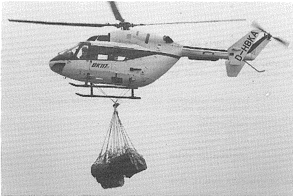
FIG. 12 Just now, the exterior sling capability of the BK 117 is being extended to 1 200 kg.
