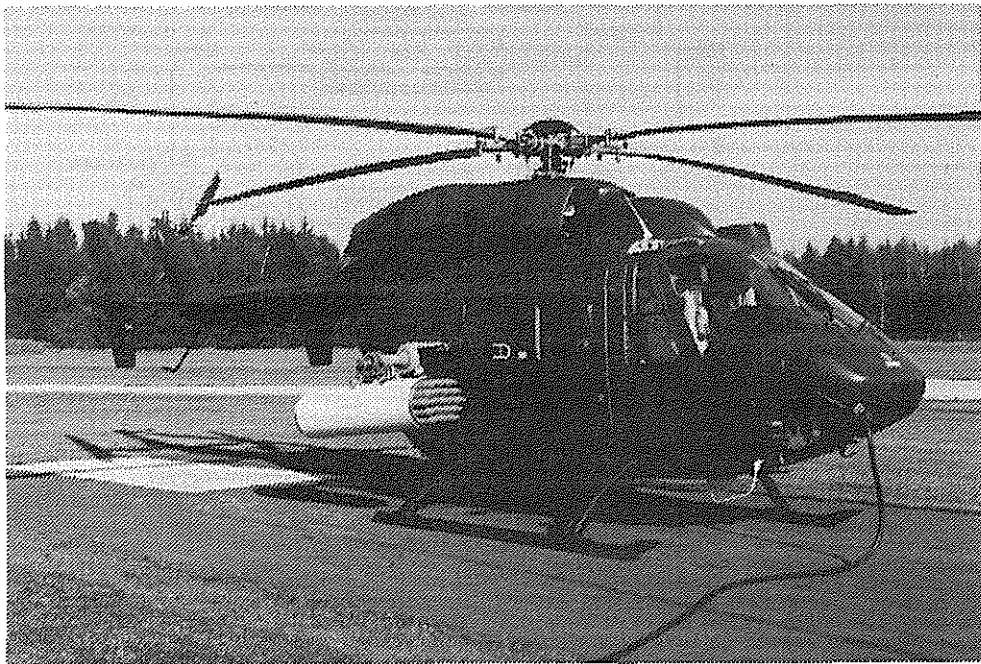
FIG. 15 BK 117 M Flight test with unguided rockets
