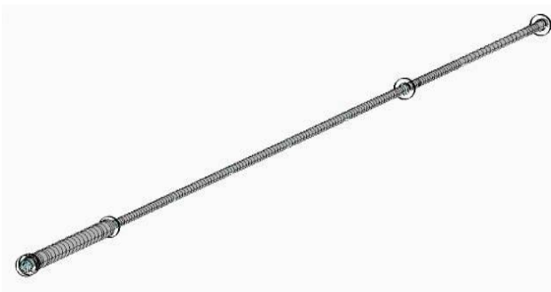
Figure 17: Tail drive shaft simulation model for shaft bending modal analysis (FE model / NASTRAN)
