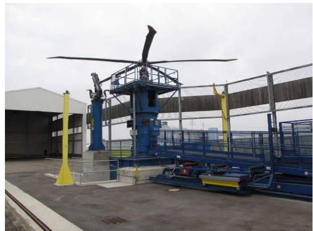
Figure 10: BLUECOPTER DEMONSTRATOR rotor on the whirltower
