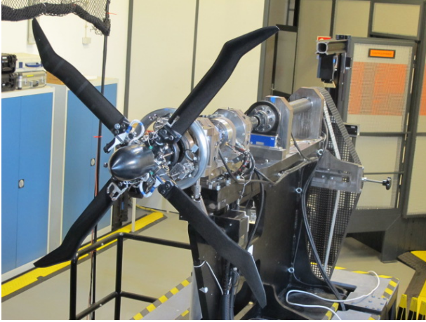
Fig. 1: Rotor Test Facility Göttingen with four-bladed rotor
