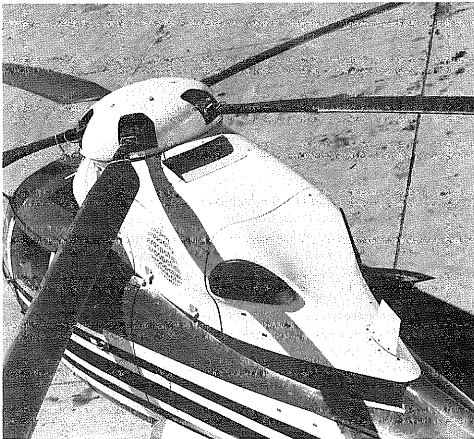
Figure 19 View of MGB compartment ventilation outlet on aircraft
