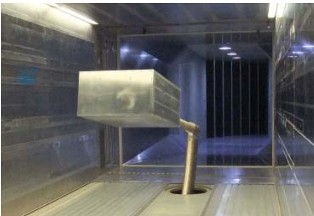
Fig. 1: The DLR F20 model in the DNW-NWB
