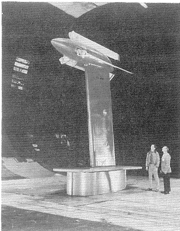
Figure 14. Bell's tilt fold rotor test in NASA's 40- by 80-foot wind tunnel.
