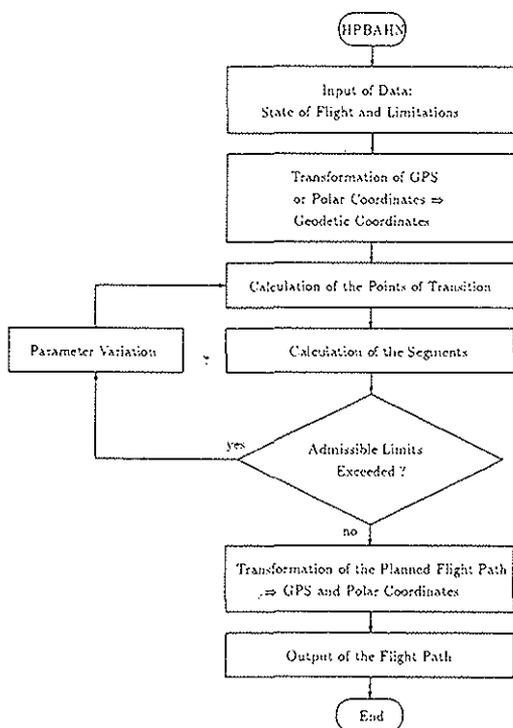
Figure 10: Flight Path Planning Algorithm HPBAHN
