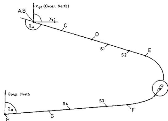
Figure 9b: Segmentation of the Approach Path in the Horizontal Plane
