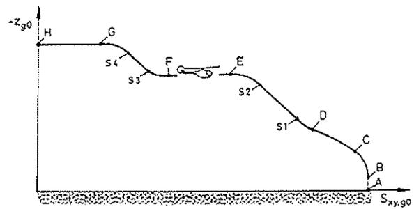
Figure 9a: Segmentation of the Approach Path in the Vertical Plane
