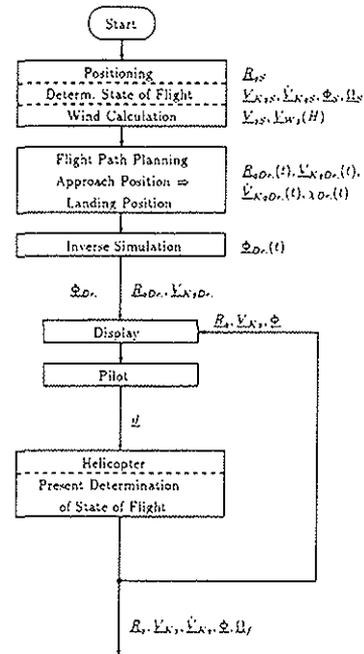
Figure 12: Pilot Controlled Approach Concept
