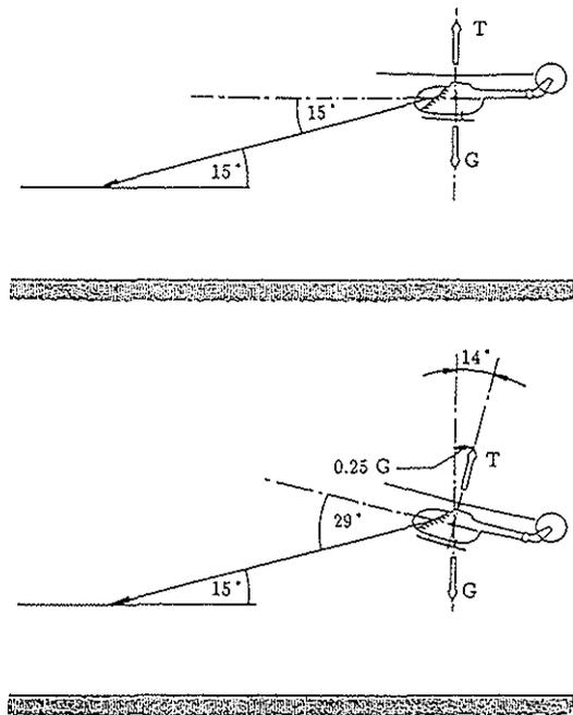
Figure 3: Visual Angle of Stationary and Decelerated Steep Approach
