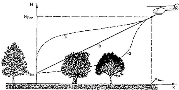
Figure 2: Steep Approach on Straight Lined or Curved Flight Path
