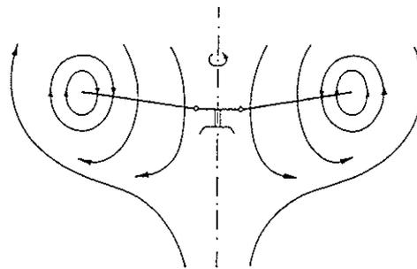
Figure 6: Vortex Ring State in Vertical Descent
