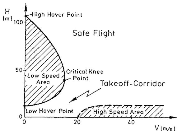
Figure 5: Height-Velocity Diagram
