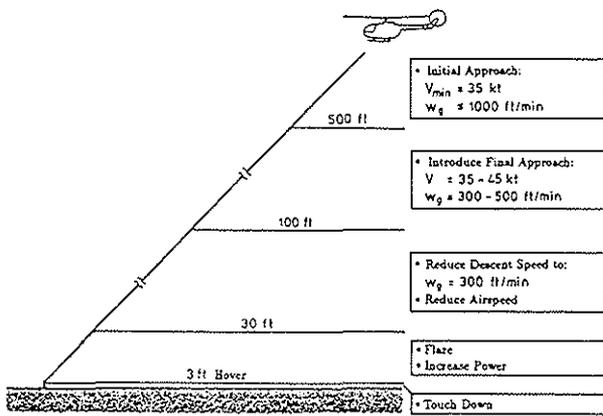
Figure 1: Steep Approach in Reference to the BO 105 Flight Manual [1]
