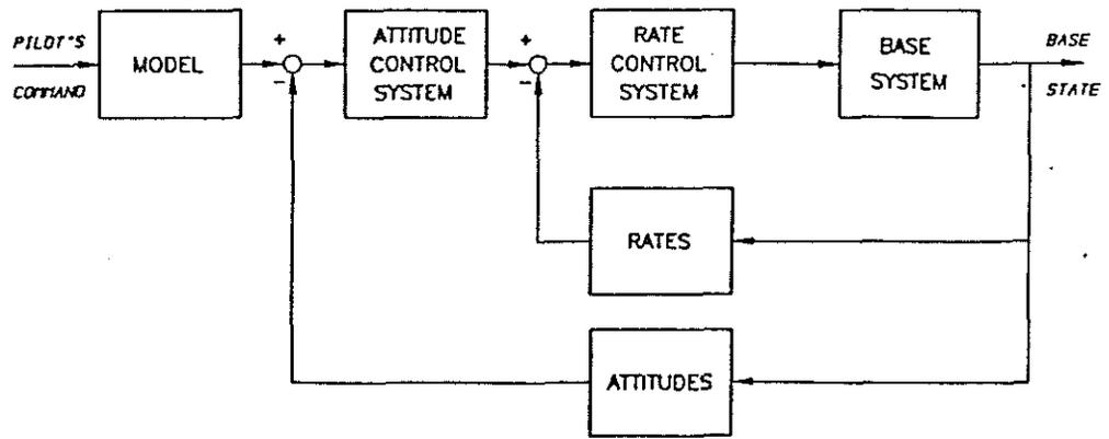
Figure 9 Model Following Control System
