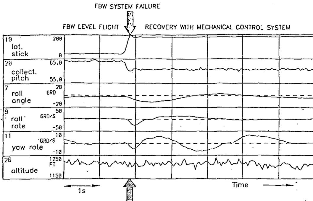
Figure 6 Fly-by-Wire Actuator Runaway
