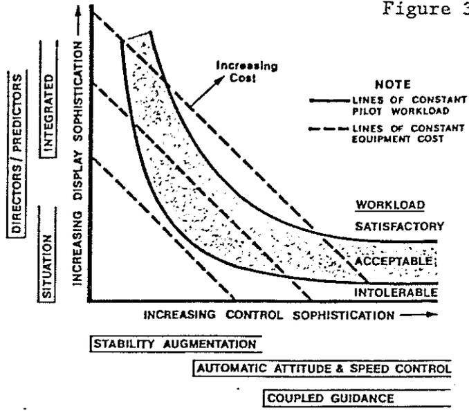
Figure 4 Hypothesis for Control System/Display Tradeoff
