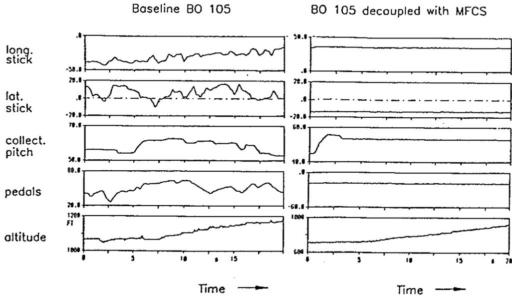
Figure 13 Comparison of Pilot's Control Activity in Climb (1000 ft/min)
