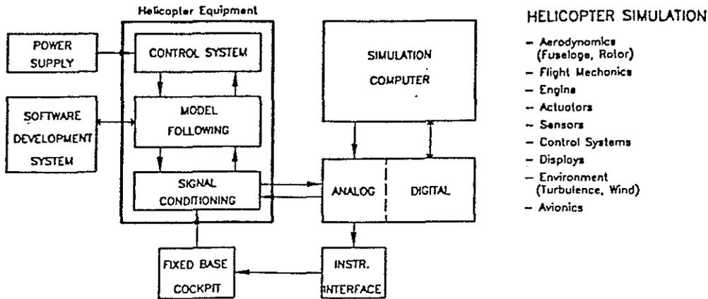
Figure 12 System Simulator for BO 105 ATHeS
