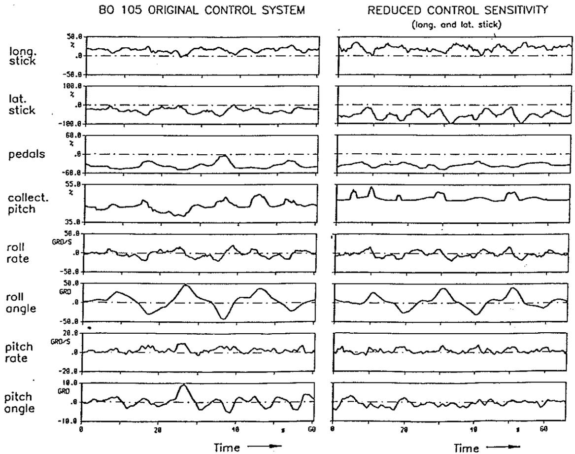
Figure 14 Effect of Control Sensitivity in NOE Slalom Task
