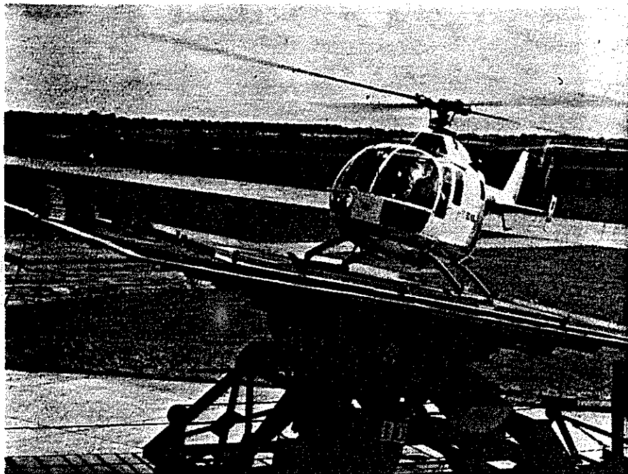
FIG. 6: BO - 105 on Rolling Platform. Landing direction 45^{\circ} to roll axis
