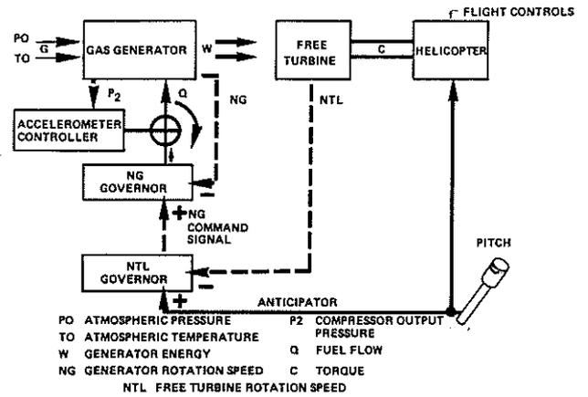
FIG. 2 : ENGINE AND GOVERNING SYSTEM - SIMPLIFIED SCHEMATIC DIAGRAM
