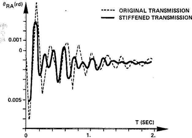
FIG. 8 : RESPONSE TO A GIVEN TAIL ROTOR TRANSMISSION TORQUE STEP
