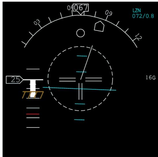
Figure 2: Symbology to be displayed on the MFD including rising deck, VSI, drift vector, acceleration cue and doghouse. The symbology is a further development of the symbology developed in the German SELA project.
