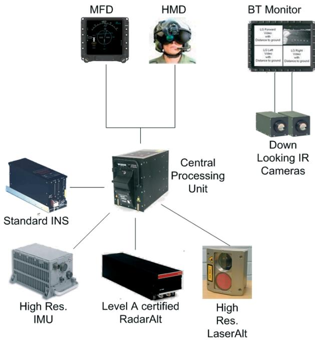
Figure 1: Architecture of the DeViLA concept in phase 1 with sensors for drift and height above ground detection.
