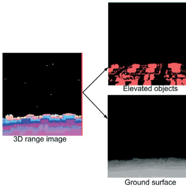
Figure 5: Separation of 3D data sets into ground surface and elevated objects. In the 3D range image distance is coded in pseudo-colors.
