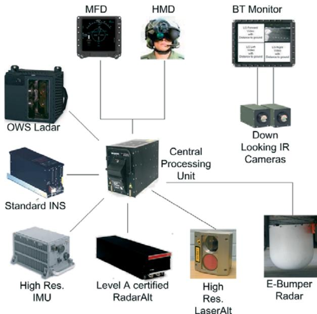
Figure 4: Architecture of the DeViLA concept in phase 3 with an additional OWS ladar sensor used as the basis for synthetic vision display.
