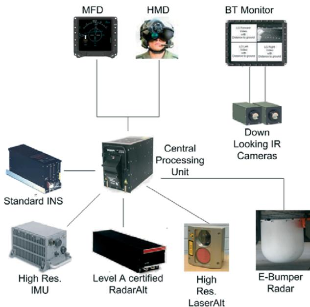
Figure 3: Architecture of the DeViLA concept in phase 2 with an additional E-bumper radar sensor.
