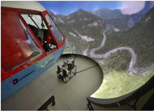
Figure 4 Ambient visual conditions emulation system
