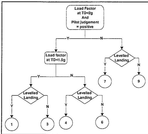
Figure 3 Score determination process
