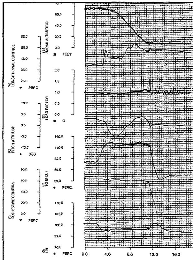
Figure 2 Emergency landing with flare
