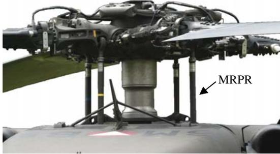
Figure 1. Rotor head of a Black Hawk helicopter.
