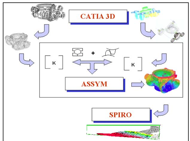
Thanks to the advances integrated in ASSYM and in design software, such as CATIA®, it is now possible in this new step to design and model all the parts in 3 dimensions, regardless of their complexity.
