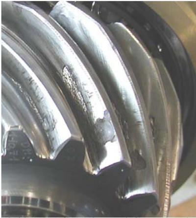
**Flaking on Spiral Bevel Gear Teeth**
