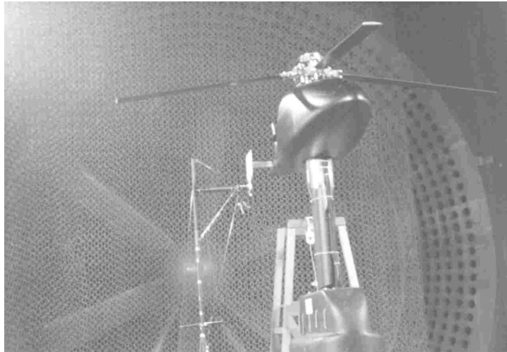
Fig. 7: HW probe support mounted on traversing pylon
