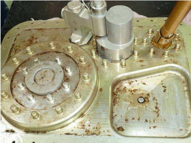
**Figure 8 Damage of a fuel equipment plate due to Bio-contamination**
