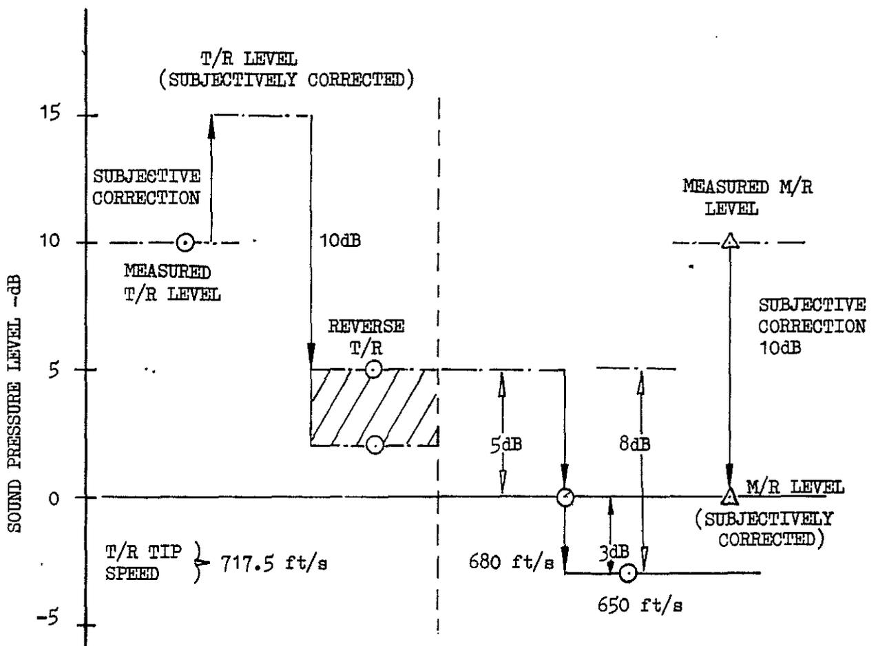
FIGURE 6 DIAGRAMMATIC REPRESENTATION OF NOISE REDUCTION ON APPROACH
