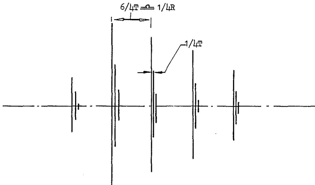
FIGURE 5 OVERHEAD INTERACTION NOISE - PULSE CHARACTERISTICS
