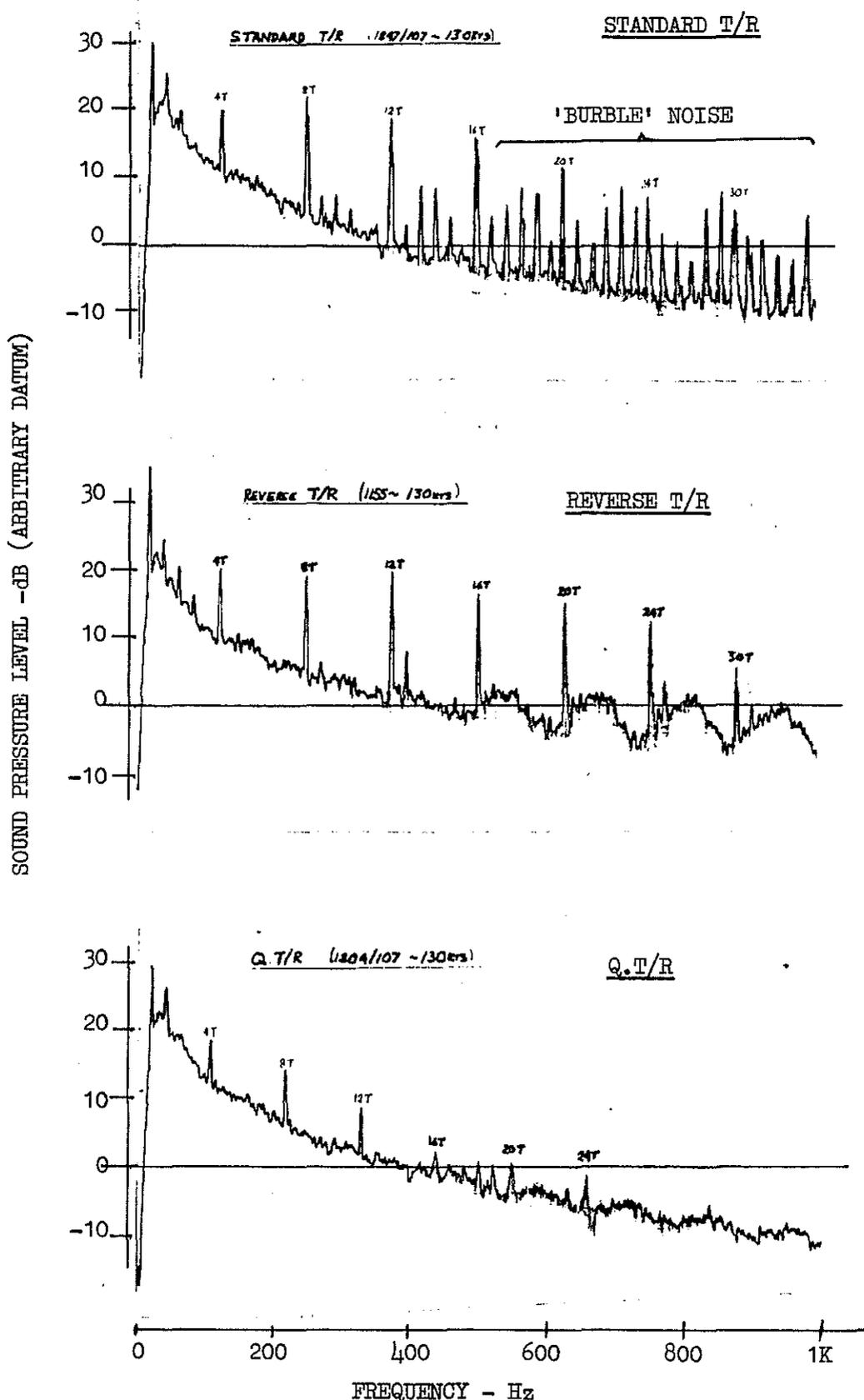
FIGURE 7 NARROWBAND ANALYSIS - TAIL MOUNTED MICROPHONE (FLIGHT SPEED 130 KNOTS)
