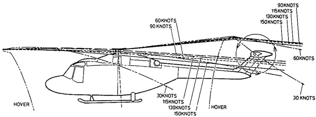
FIGURE 3 MAIN ROTOR TIP VORTEX TRAJECTORIES
