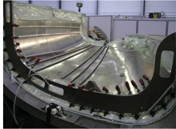
Figure 27, intermediate structure, Stringers welding.
