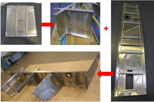
Figure 42, Beam welding sequences.
