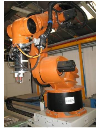
Figure 3, Kuka robot installed on a rail (7 th axe) equipped with Cytec welding head.
