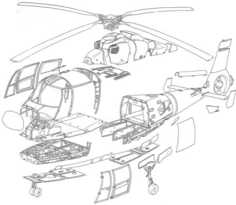
Figure 4, Main structural components of a helicopter
