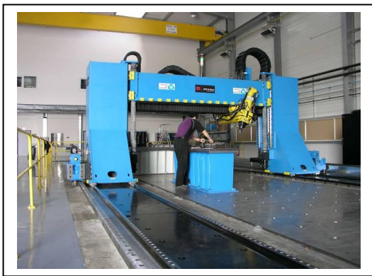
Figure 2, the specific gantry machine (5 axis mean).
