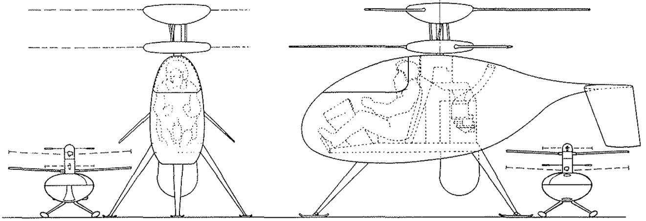
**Figure 1 Comparison of Remotely and On-Board Piloted Airborne Surveillance Systems**
