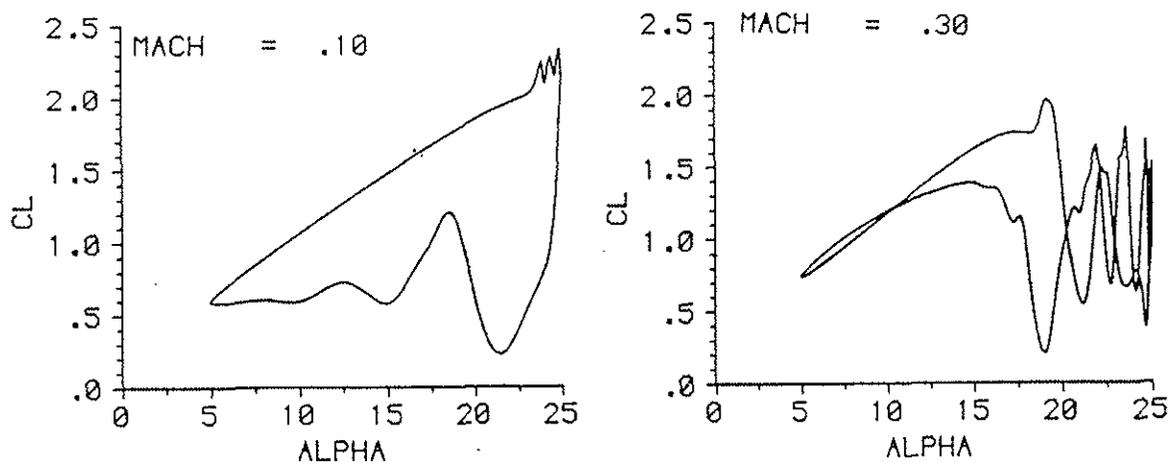
**Fig.6: Lift-distributions versus incidence:  $\alpha = 15^\circ + 10^\circ \sin \omega^* \cdot T$**
