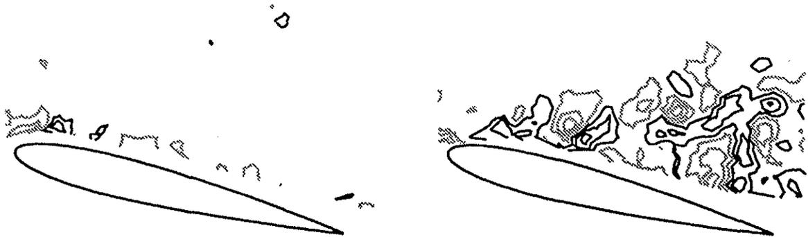
**Fig.11: Contours of  $div w$ , left:  $\alpha = 15^\circ \uparrow$ , right:  $\alpha = 15^\circ \downarrow$**
