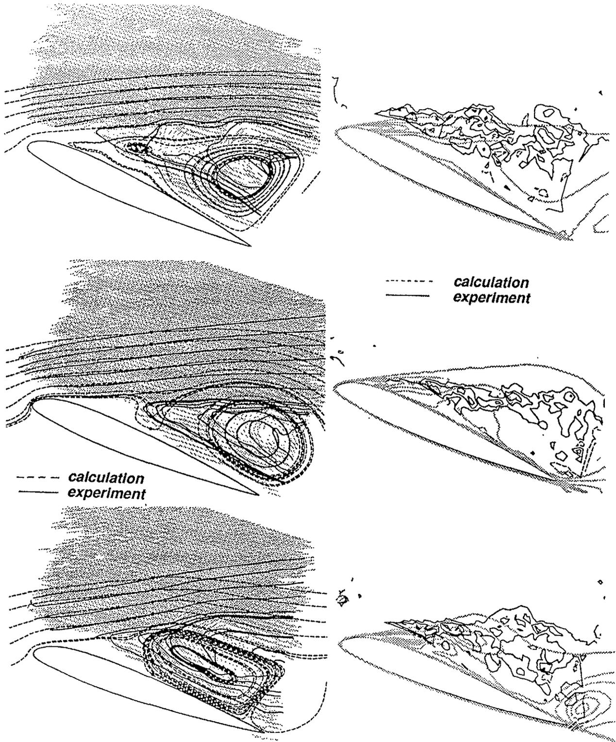
**Fig.13: Downstroke motion of NACA23012 airfoil in HKG Wind Tunnel**
