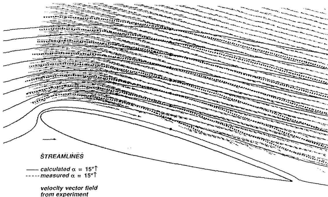
**Fig.8: Instantaneous streamlines at  $\alpha = 15^\circ \uparrow$ ,  $Re = 0.4 \cdot 10^6$ ,  $\omega^* = 0.3$**
