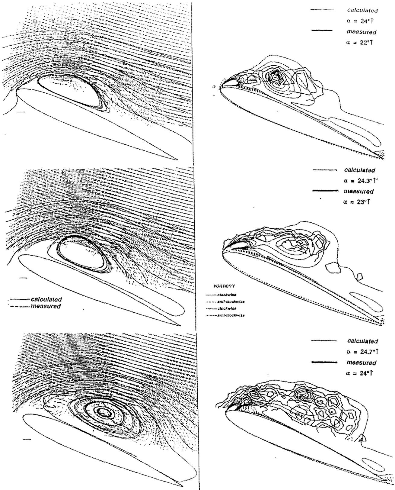
Fig.9: Upstroke motion. Streamlines (left) and vorticity contours (right) for NACA0012 airfoil in the high incidence upstroke motion: Start and movement of the dynamic stall vortex.
