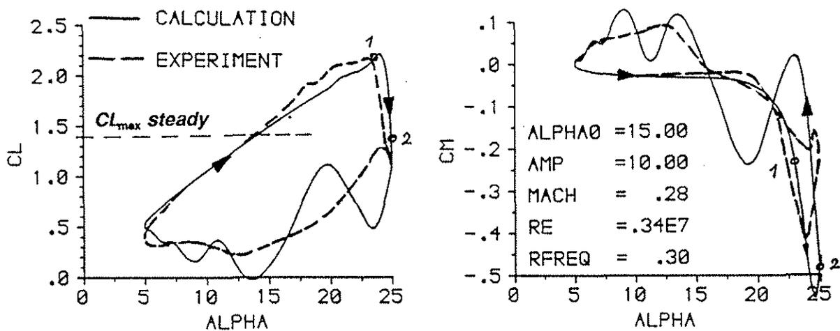
Fig.1: Lift-and moment-loops at deep dynamic stall on NACA0012 airfoil.
