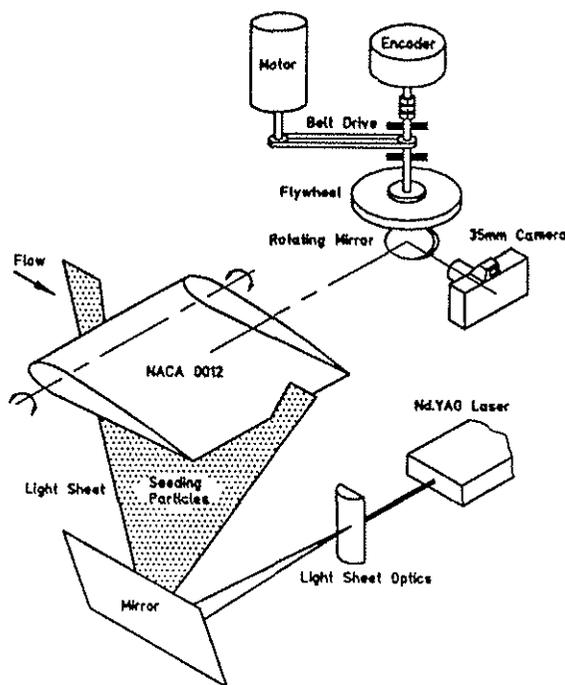
**Fig.3: Sketch of experimental set up of the PIV system in a wind tunnel.**
