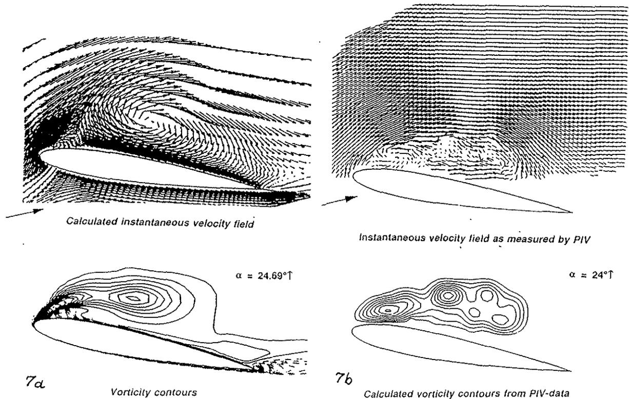
**Fig.7: Instantaneous velocity fields, vorticity contours during upstroke of NACA0012 airfoil.**
