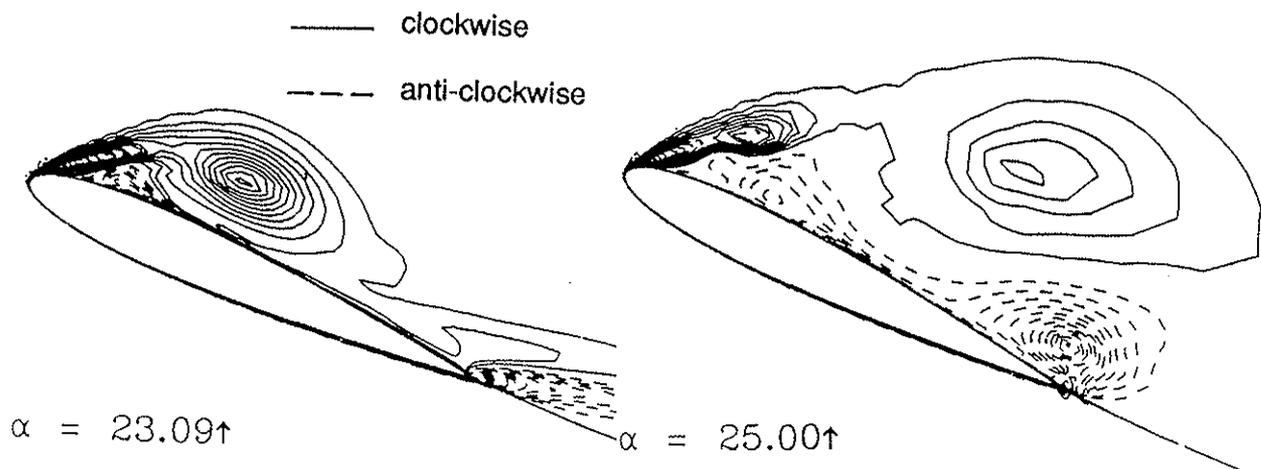
**Fig.2: Instantaneous vorticity contours on NACA0012 airfoil.**
