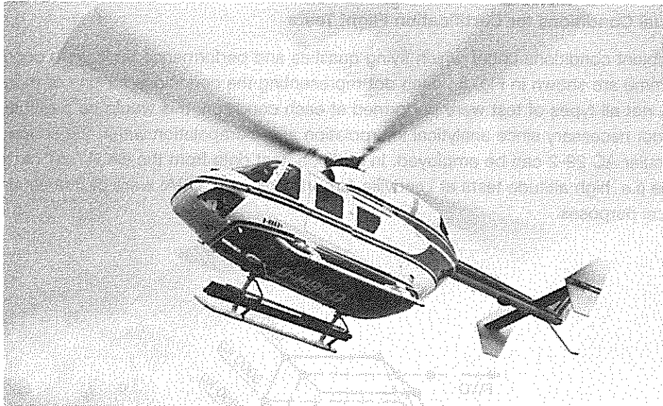
Fig. 7 BK117 with External Ballast for stb. c.g. Limit Controllability Tests at Leadville, Colorado
