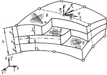
Figure 2. Multilayered finite element.
