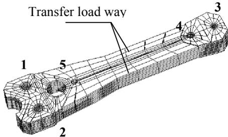
Figure 3. Finite element model of the torsion.
