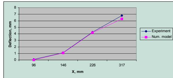
**Example 3. Bending of a torsion in rotation plane by force  $P_X=500$  N.**
