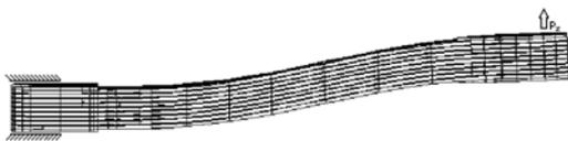
**Figure 7. Deflection curve of the torsion.**
