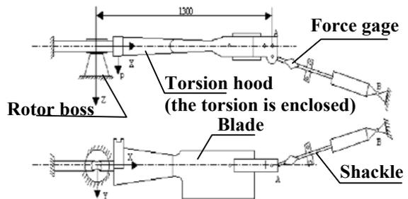
Figure 5. The test board scheme.
