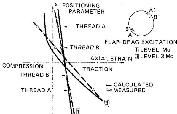
Fig. 14 : NORMAL STRESSES GENERATED BY FLEXURE
