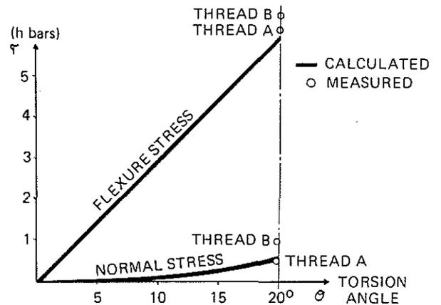
Fig. 15 : NORMAL STRESSES GENERATED BY TORSION
