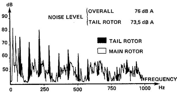
Fig. 23 : IMPORTANCE OF TAIL ROTOR NOISE IN HELICOPTER RADIATION
