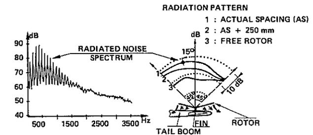
Fig. 25 : TAIL BOOM AND FIN INTERACTION EFFECT ON NOISE
