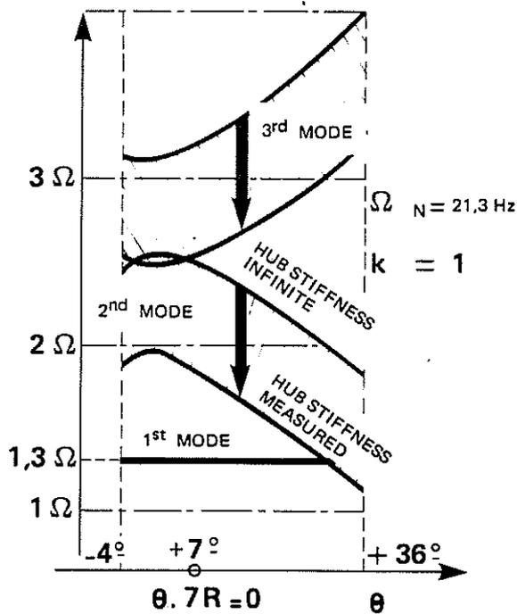
Fig. 7 : INFLUENCE OF PITCH AND HUB STIFFNESS ON NATURAL FREQUENCIES
