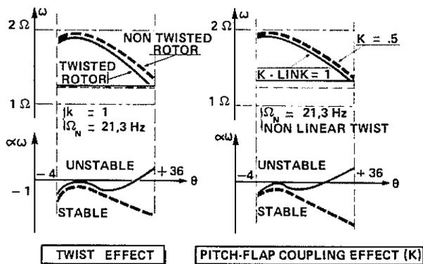
Fig. 8 : INFLUENCE OF TWIST AND PITCH-FLAP COUPLING ON NATURAL FREQUENCIES AND DAMPING
