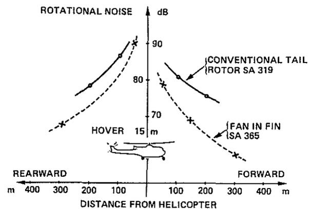
Fig. 29 : EXTERNAL NOISE COMPARISON
