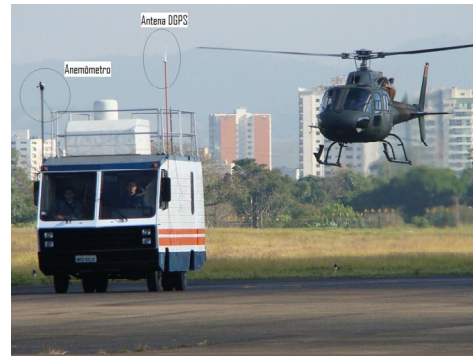
Figure 1 - Picture of Pace Car Flight Test Method.
