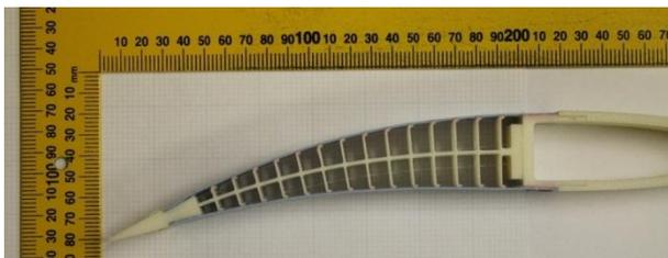
Fig. 6 FishBAC internal structure
