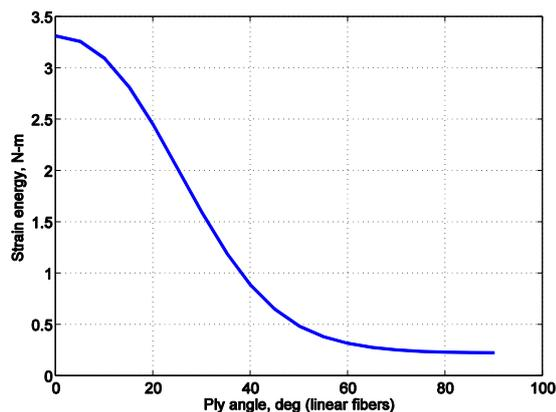
Fig. 10 Strain energy of skin due to camber variation
