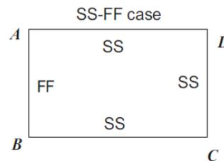
Fig.3b Out-of-plane loading boundary conditions
