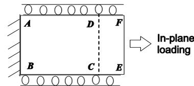
Fig.3a In-plane loading boundary conditions
