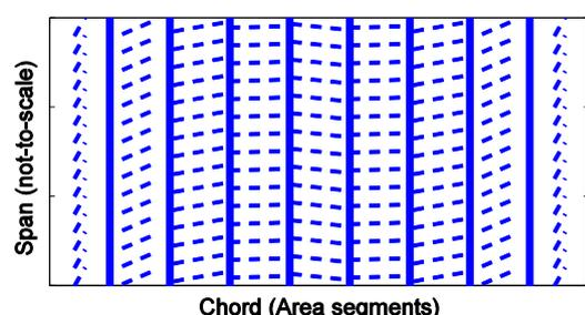
Fig. 5 Variation of FR of the plate with curved fiber paths and the optimal fiber paths for aspect ratio 2.0
