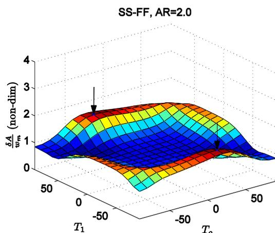
Fig.4 Variation of FR of the plate with curved fiber paths and the optimal fiber paths for aspect ratio 2.0
