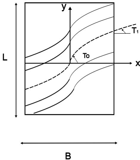
Fig.1 Curved fiber composites
