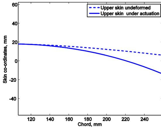
Fig. 9 Upper skin deformations under actuation forces
