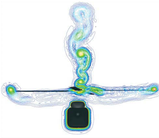
Figure 7: Vorticity magnitude at \psi = 0^\circ and x/l = 0.9 for \mu = 0.15 and C_T = 0.0064 .
