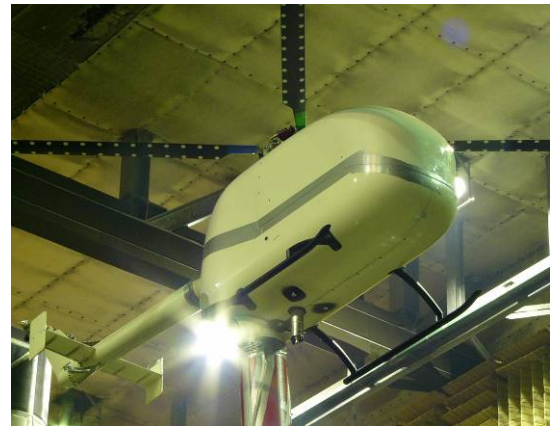
Figure 6: Model with modified fuselage contour
