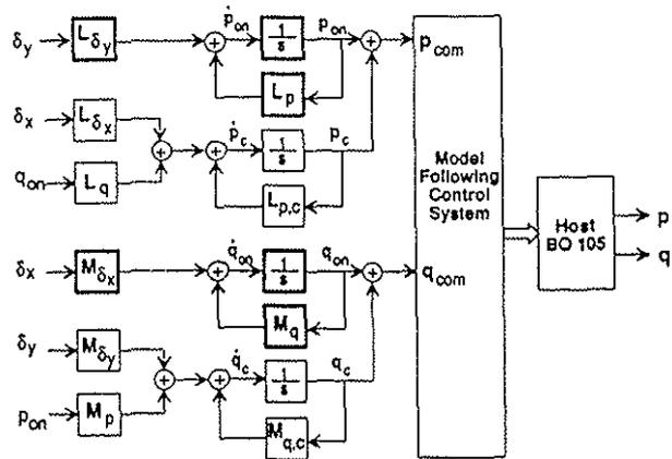
Figure 6. Models of pitch and roll axis
