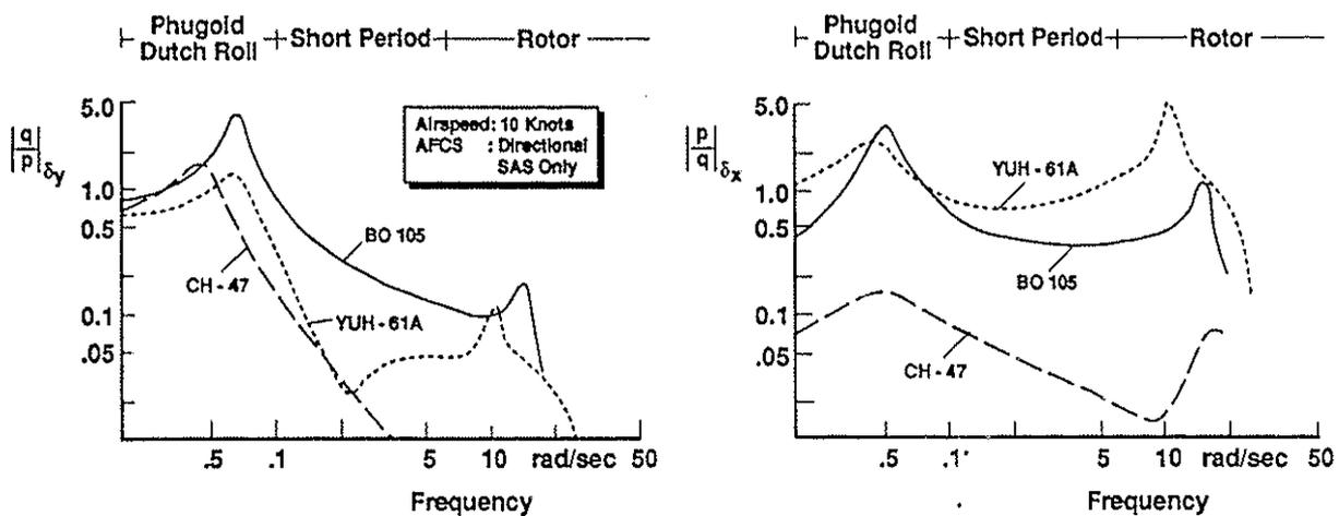
Figure 1. Frequency dependency of pitch-roll cross coupling (ref. 1)
