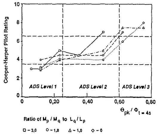
Figure 10. Pilot ratings versus  $\theta_{pk} / \phi$  for varied roll-to-pitch and pitch-to-roll ratios
