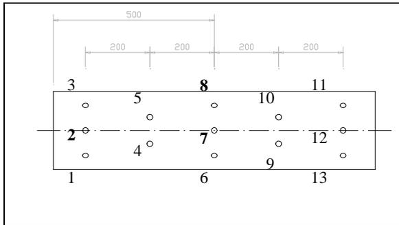
**Figure 7 Pressure transducers: identification number and location.**
