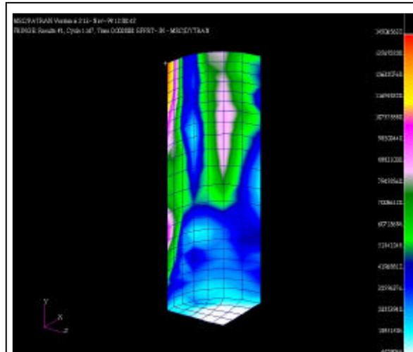
**Stress on the surface of the specimen – calculated using MSC/Dytran.**
