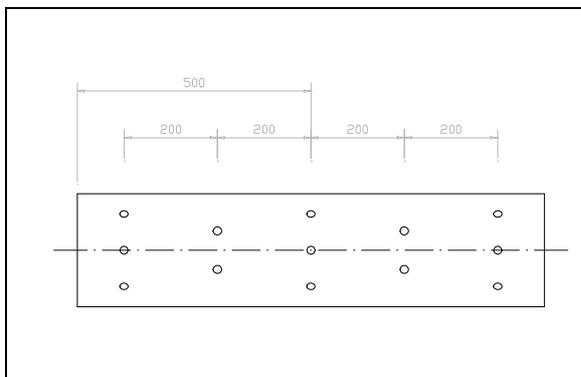
**Figure 2 Location of the pressure transducers.**
