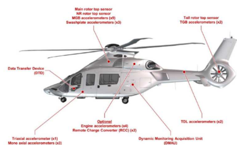
Figure 3: MR and TR magnetic tops
