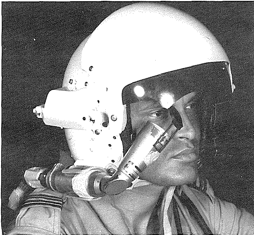
Fig 5 Trials helmet and HMD
