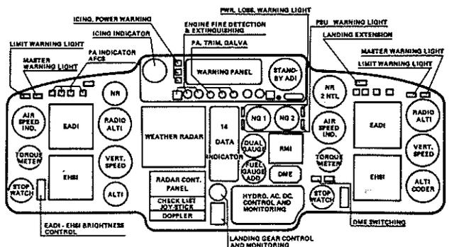
Fig. 11 SA 365 F INSTRUMENT PANEL MULTIFUNCTION DISPLAY CONFIGURATION
