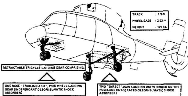
**Fig. 3 SA 365 F LANDING GEAR**
