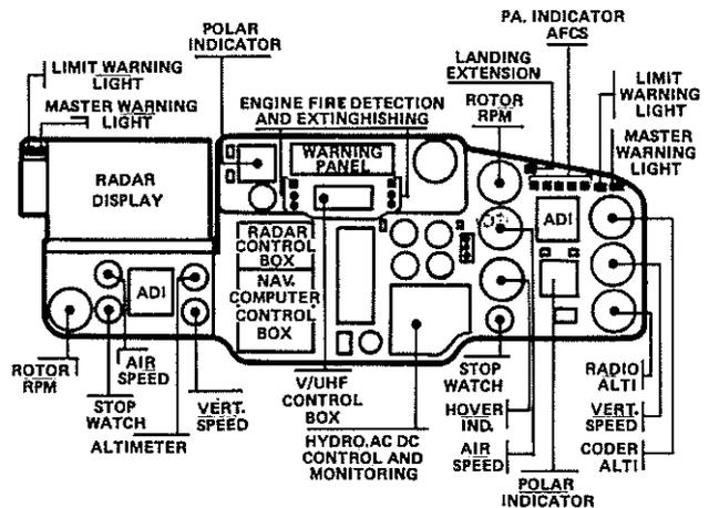
Fig. 10 SA 365 F INSTRUMENT PANEL ELECTRO- MECHANICAL FLIGHT INSTRUMENTS
