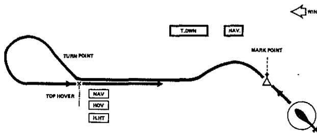
Fig. 7 APPROACH OF A MARKED POINT
