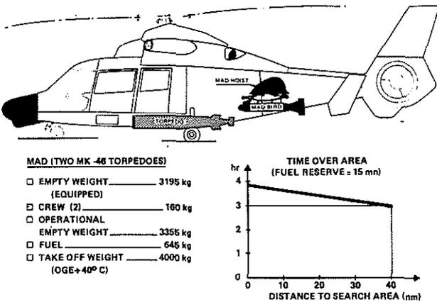
Fig. 24 MAD - TORPEDOES INSTALLATION
