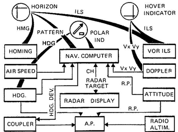
Fig. 9 SA 365 F SAR SYSTEM- INTERCONNECTION- CONVENTIONAL WIRING
