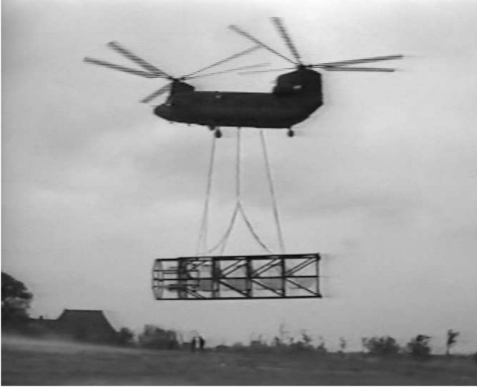
Figure 1. Picture of the tandem-suspension external load under tandem-rotor helicopter.
