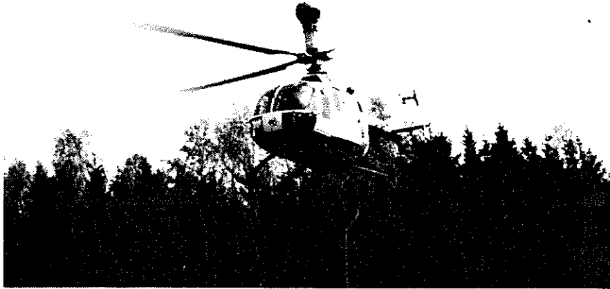
Fig. 1: Bo 105 with platform mock up (90 cm rotormast extension)
