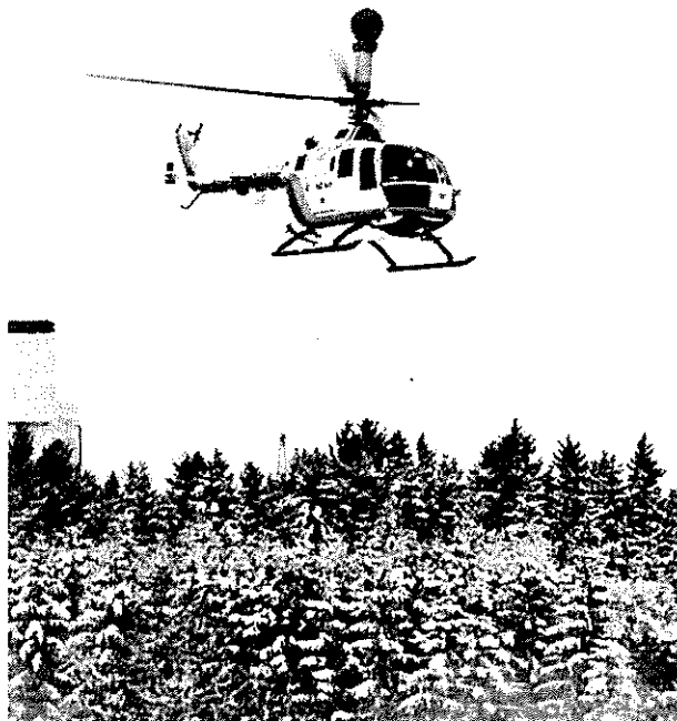
Fig. 2: Bo 105 with platform mock up (120 cm rotormast extension)
