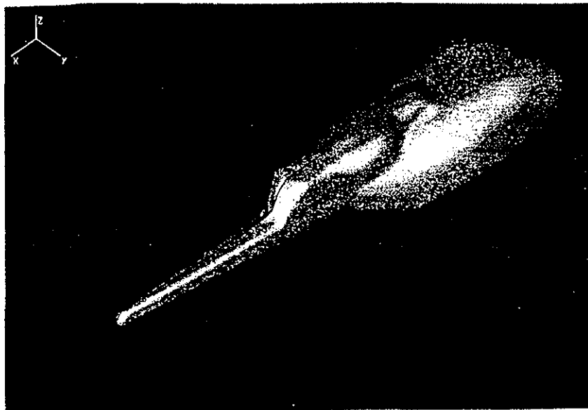
Figure 3: Alouette III fuselage and cowl surface as obtained from CAD.
