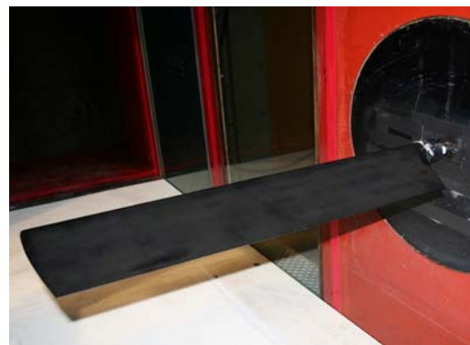
Figure 1: View of the OA209 wing model in the F2 wind-tunnel
