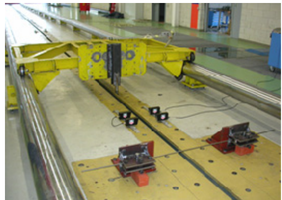
Figure 8. The horizontal sled and the test facilities used in the dynamic tests.
