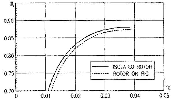
FIGURE 16 : EFFECT OF THE TEST RIG INTERACTIONS (CALCULATED)
