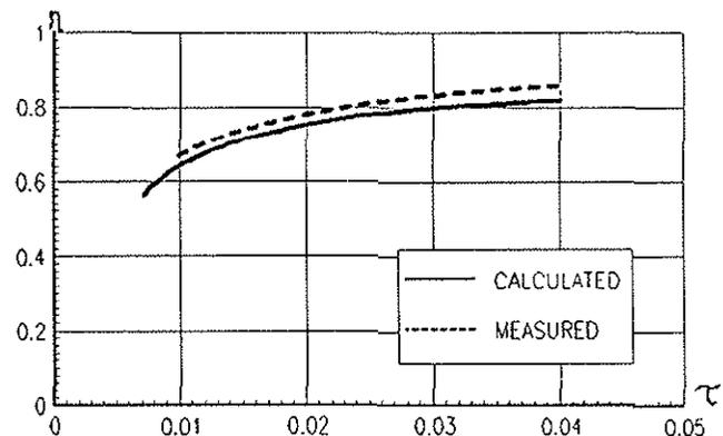
FIGURE 12 : EFFICIENCY AT M = 0.5 VERSUS THRUST COEFFICIENT
