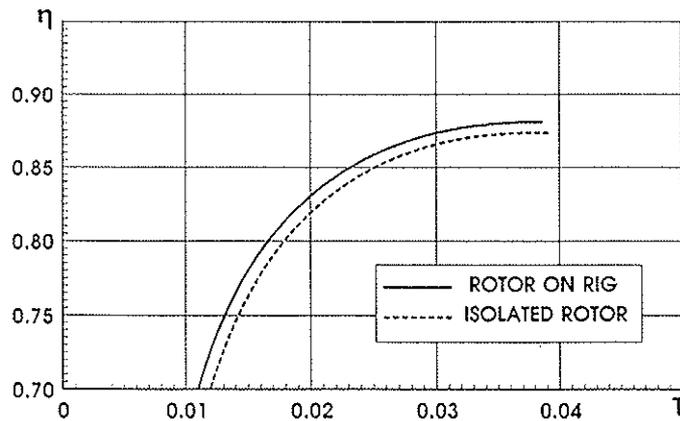
FIGURE 16 : EFFECT OF THE TEST RIG INTERACTIONS (CALCULATED)
