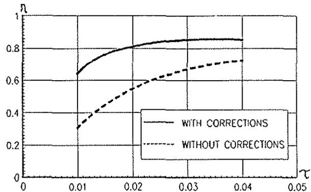
FIGURE 11 : ROTOR EFFICIENCY EFFECT OF THE CORRECTIONS
