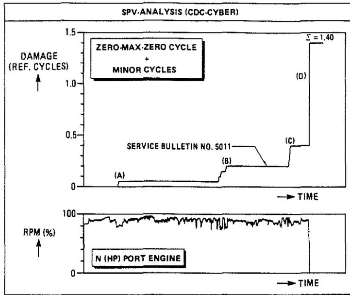
Fig. 9 Port engine damage accumulation during flight no. 3
