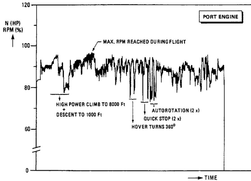
Fig. 8 RPM-time history port engine N (H) (flight no. 3)
