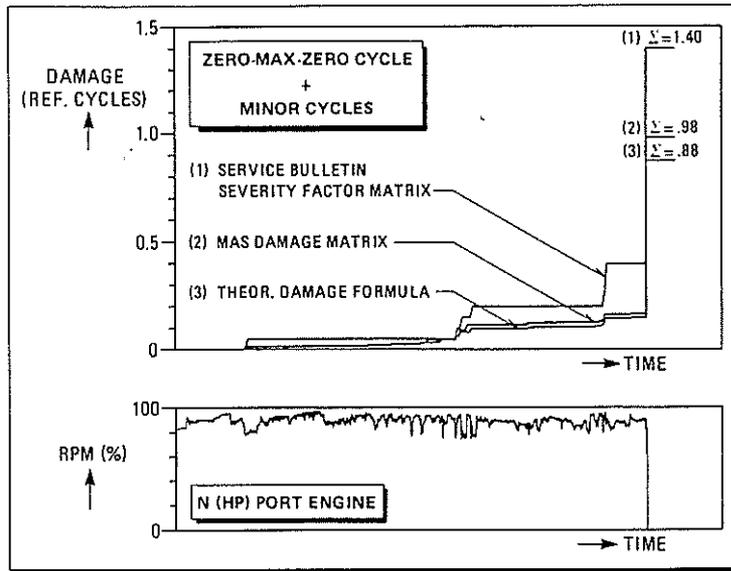
Fig. 11 Comparison of the various damage calculation procedures
