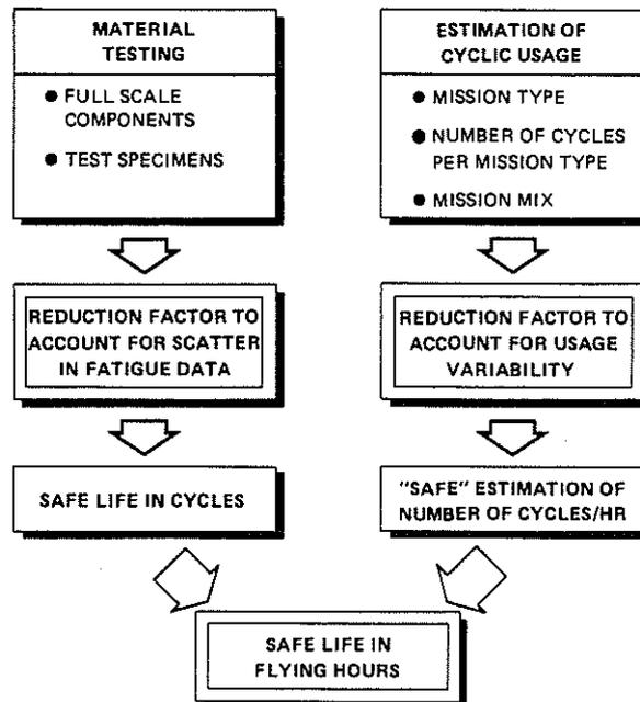
Fig. 3 Engine component lifing procedure
