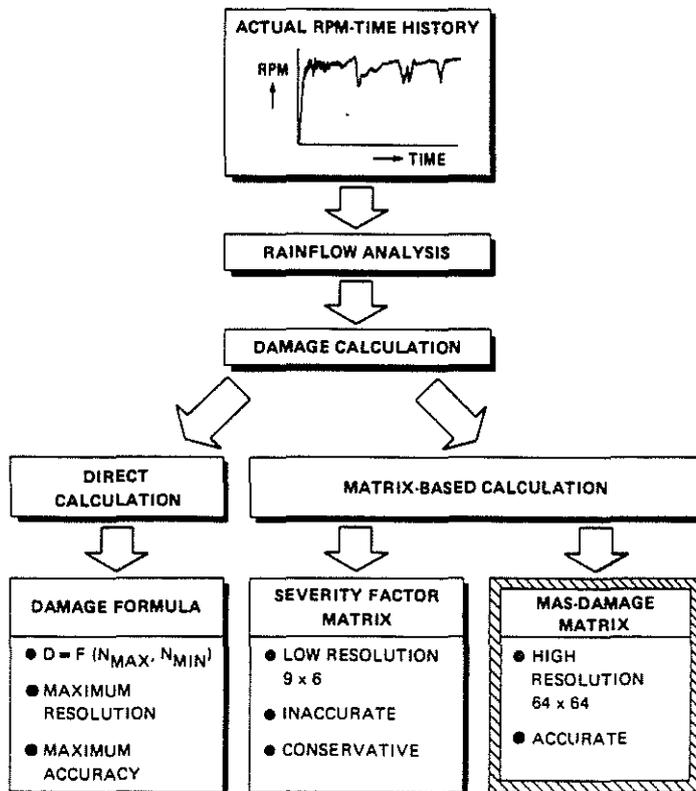
Fig. 10 Refined damage calculation
