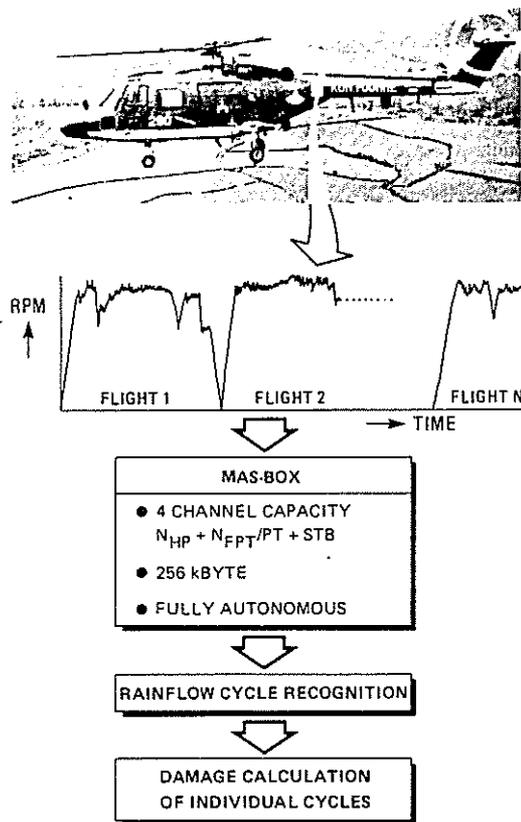
Fig. 12 Automated cyclic life control within the RNLN
