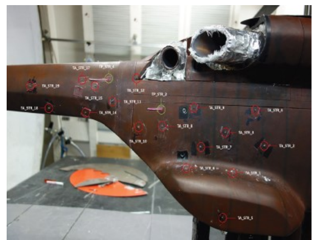
Figure 10: Visualization of the location of thermocouples on the right side of the fuselage of the helicopter mock-up.
