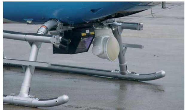
Fig. 2. Installation of the sensor-suite, first mounting onto EC135
