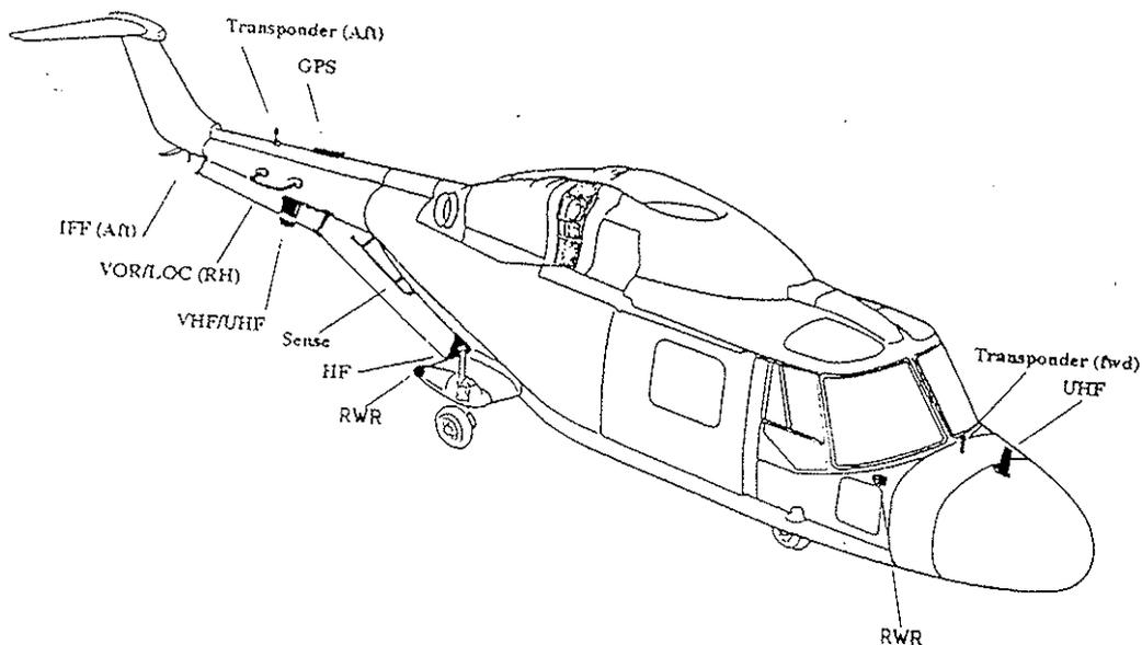
Figure 3: RNLN Lynx new antenna layout
