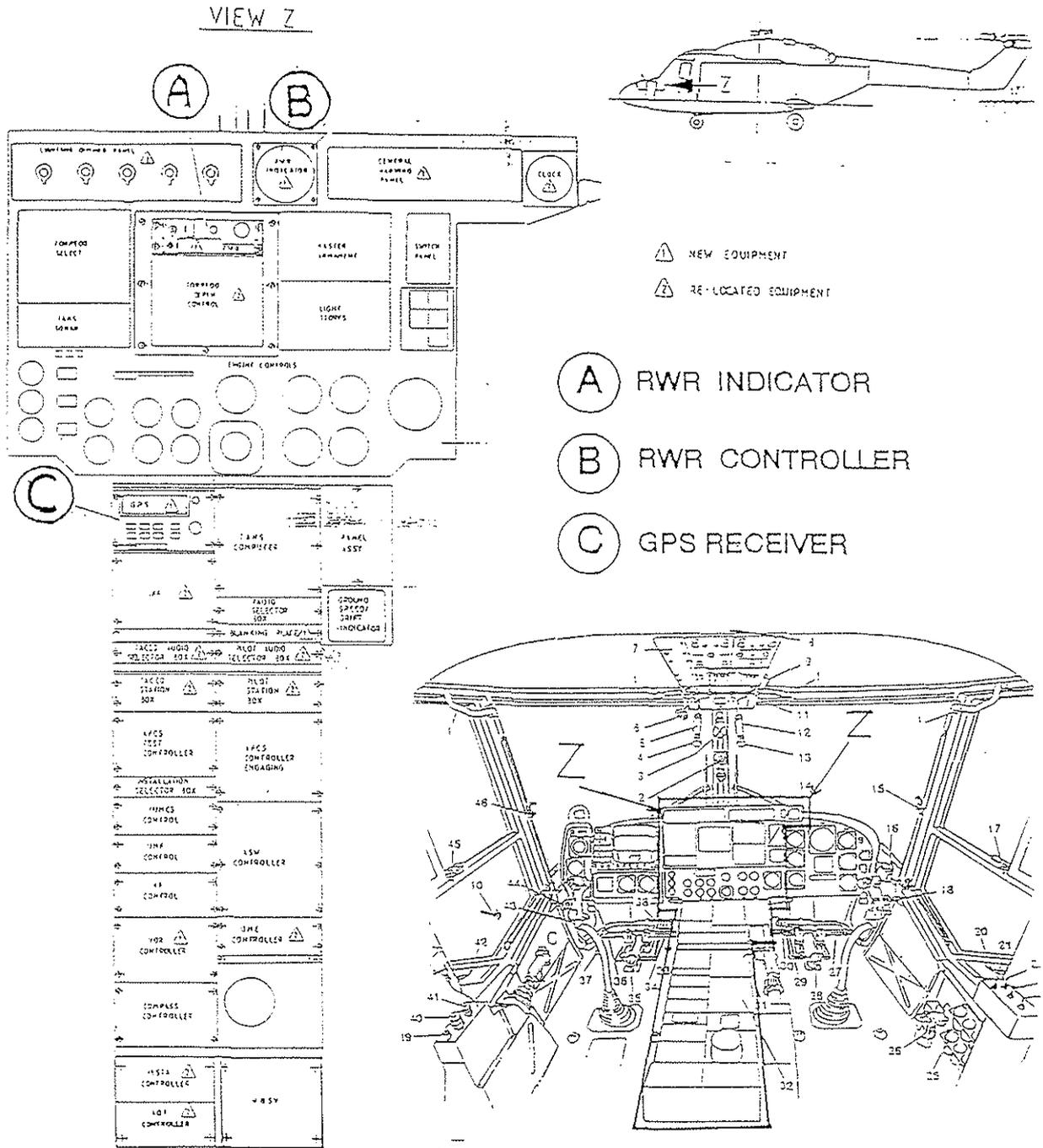
Figure 2: RNLN Lynx cockpit configuration (View Z is the new situation)
